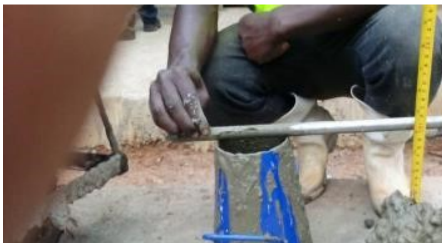
Figure 2-33: Slump test for concrete experiments
