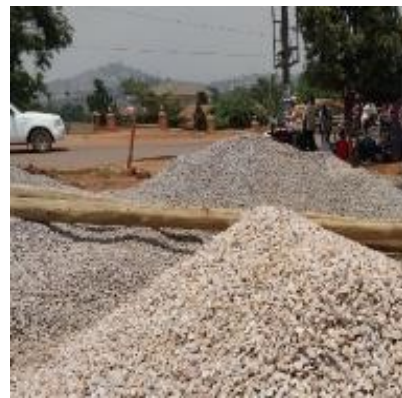
b) Kampala (Mengo): Machine crushed, Well graded aggregates from Muyenga
