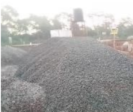
a) Luweero: Machine crushed, Well graded aggregates from Zirobwe
