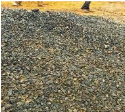
c) Fort Portal: Machine crushed, Well graded aggregates from Kasese
