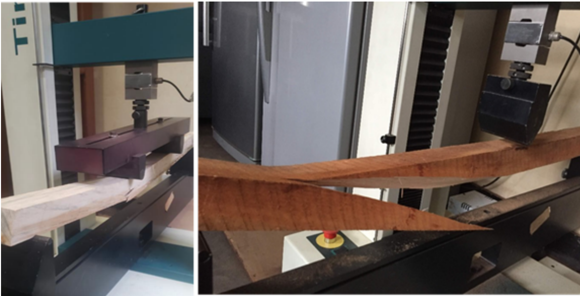
Figure 2-30: UTM Ste up for 4-point and 3-point loading test
