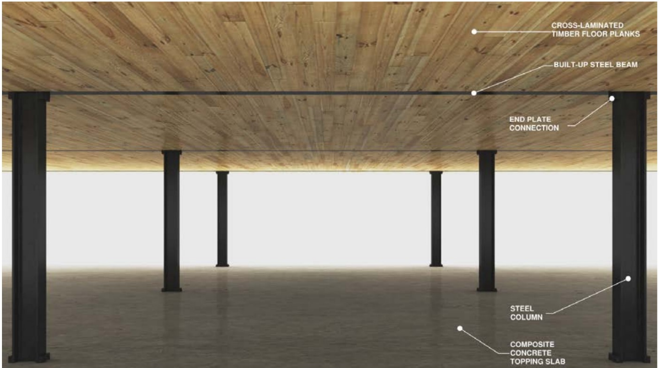
Figure 3-1: Steel-CLT timber system soffit (Credit: AISC, 2017)
