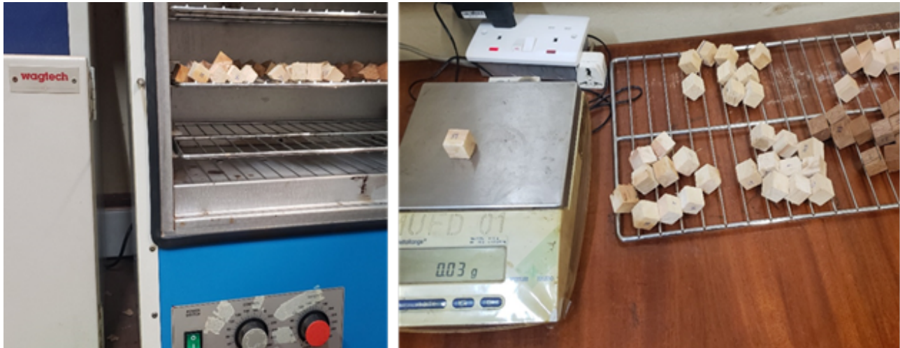
Figure 2-28: Moisture content determination using the oven dry method setup
