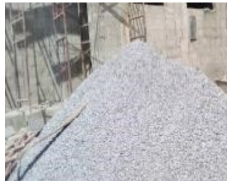
d) Lira: Machine crushed Well graded, aggregates from AFRICAN CONMAT
