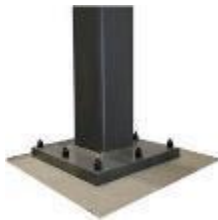
(a) Photos of unstiffened base plate
