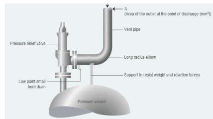
Figure 4: Illustration of Safety valve Installation on the boiler (Spirax-Sarco Limited)
